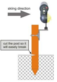
For the Transmitter-Receiver Type the Transmitters of the photocell can be either on the same side or opposite side (see manufacturer specifications). The beams may be installed in a crossed configuration but in all cases the 20cm maximum vertical separation must be observed.
